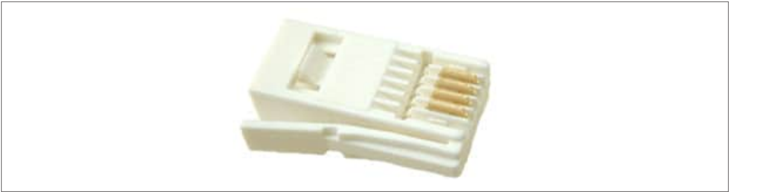
Figure 9-4. The BT plug used for analog PSTN connections in the UK (note only pins 2–5 are present)
