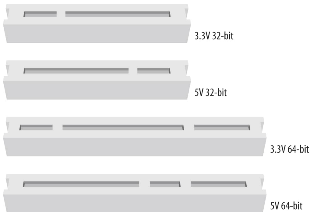
Figure C-1. Visual identification of PCI slots
