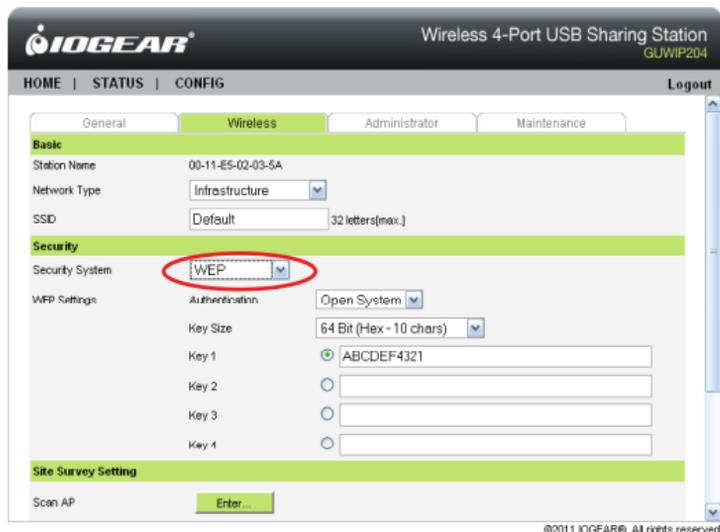
The screenshot displays the configuration interface for an IOGEAR Wireless 4-Port USB Sharing Station (GUWIP204). The page is titled "Wireless 4-Port USB Sharing Station" and "GUWIP204". The navigation menu includes "HOME", "STATUS", and "CONFIG". The "CONFIG" section is active, and the "Wireless" tab is selected. The "Security System" dropdown menu is highlighted with a red circle and set to "WEP".
