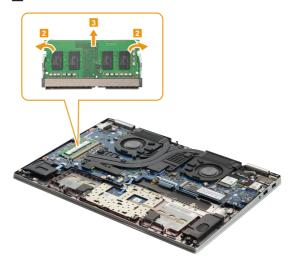
**When installing:** Insert the notched end of the DIMM into the socket. Push the DIMM firmly, and pivot it until it snaps into place. Make sure that it is firmly fixed in the slot and is difficult to move.
