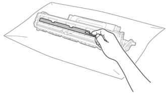
6. Put the toner cartridge back into the drum unit until you hear it lock into place. If you put the cartridge in correctly, the lock lever on the drum unit will lift automatically.
