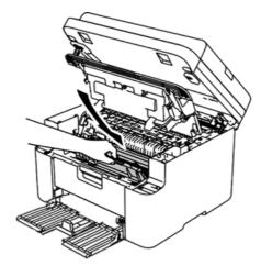
8. Close the top cover. After pulling the pull-arm (1) on the left side of the machine down, close the scanner cover using both hands.
