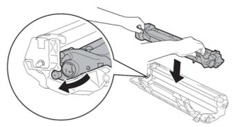
7. Put the drum unit and toner cartridge assembly back into the machine.
