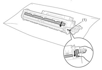
5. Wipe the surface of the drum gently with a dry cotton swab until the dust of glue on the surface comes off.
