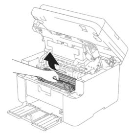
3. Push down the lock lever (1) and take the toner cartridge out of the drum unit (2).
